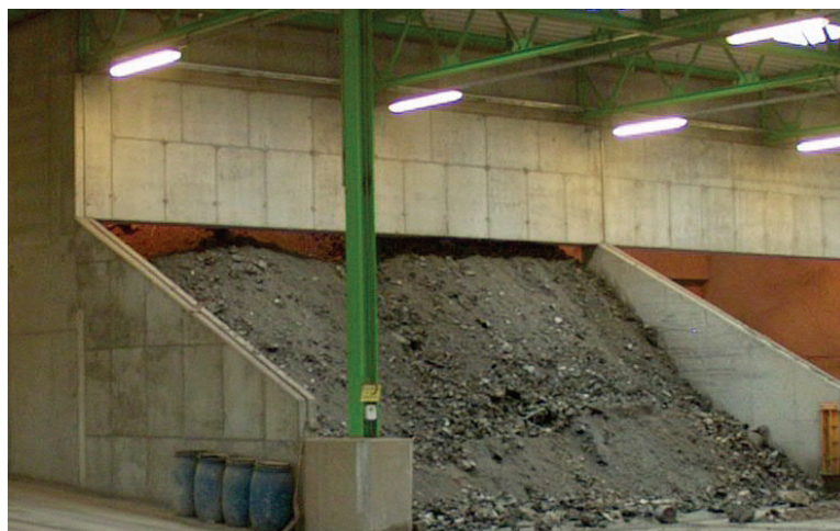
Figure A5.2 From Elsam Odense WtE – Bottom ash with a gravel-like structure
